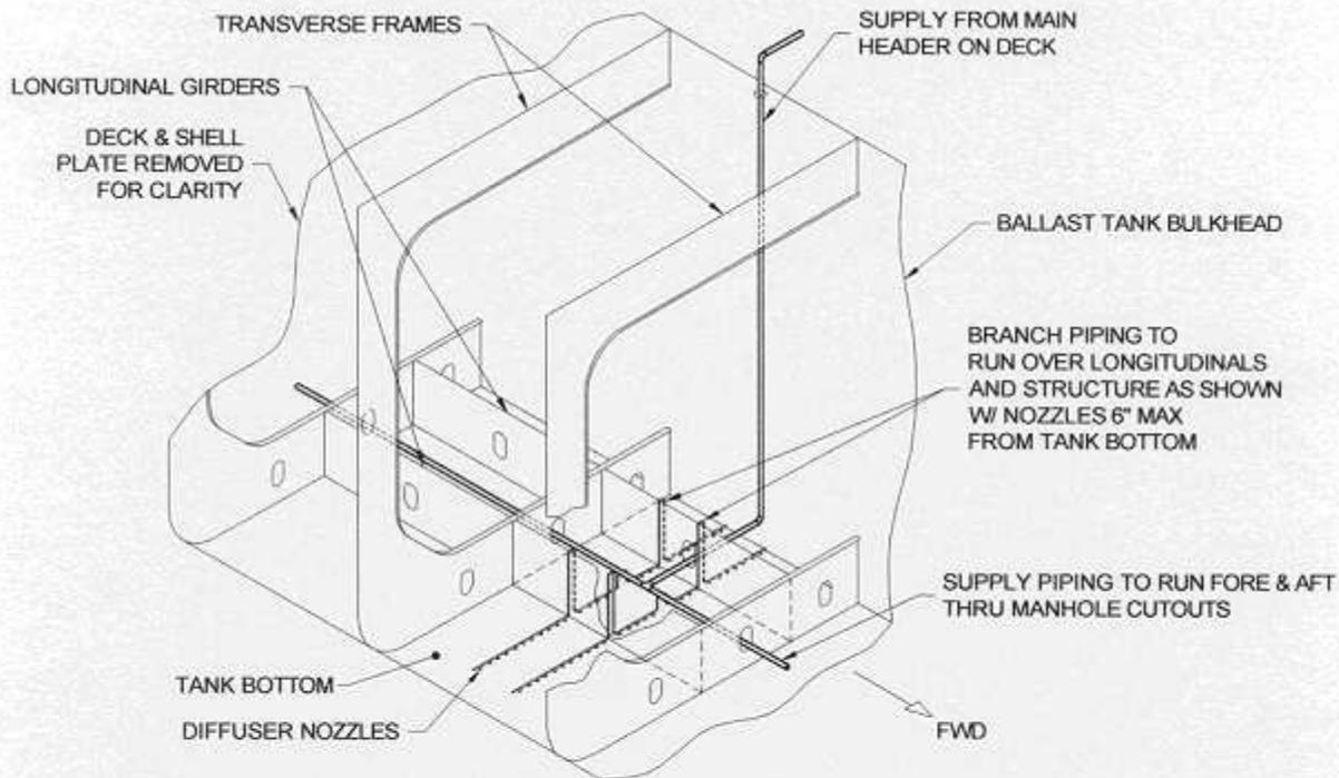
NOTE: FIG.4 DEPICTS TYPICAL BALLAST TREATMENT PIPING IN AS SINGLE HULL TANKER SEGREGATED BALLAST TANK
